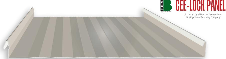
Cee-Lock — is ideal for residential or commercial construction with solid sheathing or open purlins, and features an available patented vinyl weatherseal and an integral snap-lock seam. Available in 23 standard colors and 8 premium colors. Vinyl weatherseal recommended for slopes 3:12 or less, and required for all Watertight Warranty projects.
