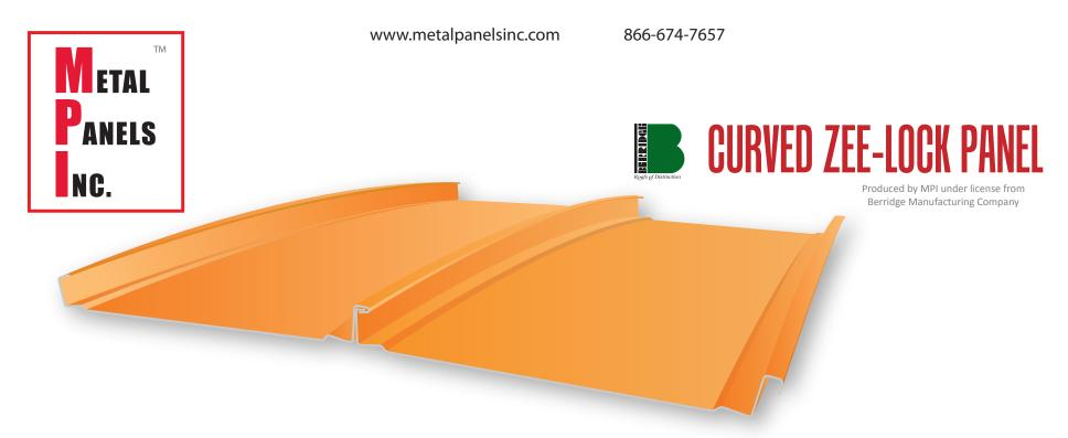
Curved Zee-Lock — is an architectural/structural mechanically-seamed standing seam roof system for use over open purlin framing or over a solid deck. Zee-Lock can be curved for radiused roof applications, with a minimum radius of 20 ft. Available in 23 standard colors and 8 premium colors. Vinyl weatherseal recommended, and required for all Watertight Warranty projects.
