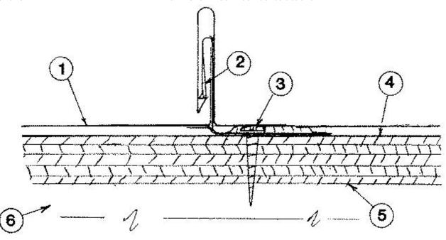
1. **Metal Roof Deck Panels\*** — No. 24 MSG min coated steel panels, max 20 in. wide, min 9 in. wide, 1-1/2 in. high at female side rib. Panels continuous over three or more clips with no endlaps. A bead of sealant may be used at panel side joints.
