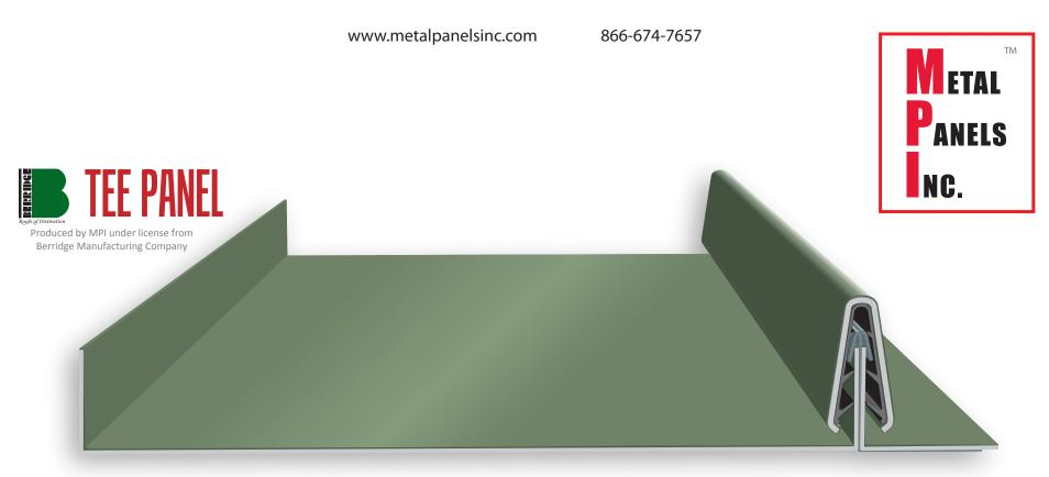
Tee-Panel – is a panel system using a snap-on seam cap with integrated vinyl weatherseal. Tee-panel is well-suited for residential or commercial construction over solid decking. Available in 23 standard colors and 8 premium colors. Minimum recommended slope is 1:12.
