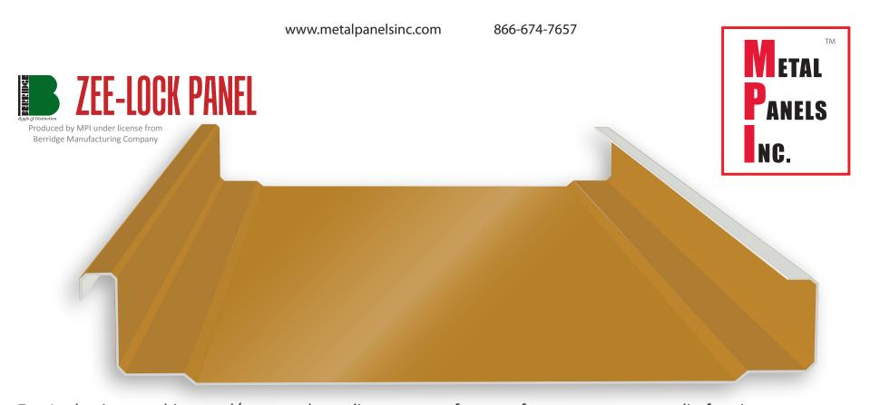
Zee-Lock — is an architectural/structural standing seam roof system for use over open purlin framing or over a solid deck. Available in 23 standard colors and 8 premium colors. Minimum recommended slope is 1:12. Vinyl weatherseal recommended for slopes 3:12 or less, and required for all Watertight Warranty projects.
