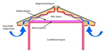
For natural air convection, the roof vents must be a minimum of three feet above the cool air intake vents. Other considerations for air flow must be followed as well. If baffled ridge vents are used, set the vent louvers against the prevailing wind direction for best weather performance. If passive roof vents are used, space evenly below the ridge line, always on one side of the roof,
