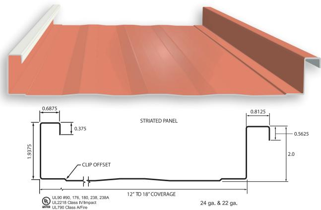
LF2A Panel -- is a mechanically-seamed architectural/structural standing seam roof system for use over open purlins or a solid deck. This panel features a return leg on both the male and female seams that help increase strength and wind uplift resistance. Minimum recommended slope is 0.5:12. Panels can be ordered as smooth, striated or two-bead.
