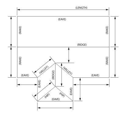
TYPICAL CURVED ROOF WITH DIMENSIONS NEEDED.
