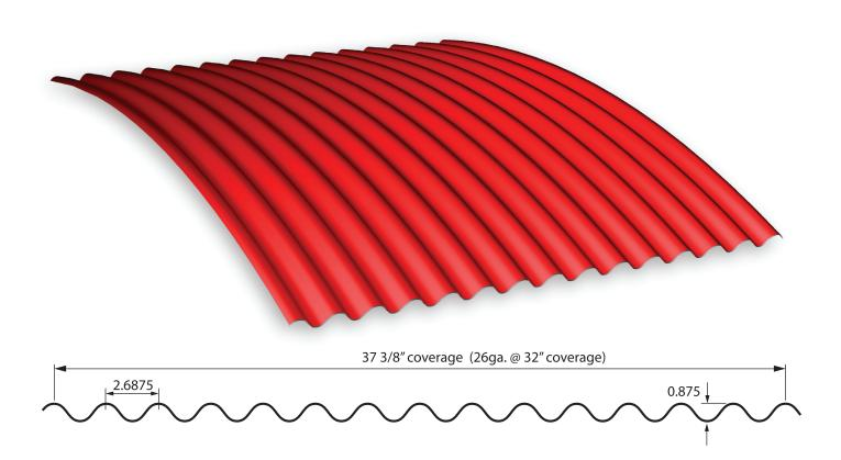
7/8" Corrugated Panel - Structurally strong and incredibly impact resistant, MPI's 7/8" Corrugated Panel is an excellent choice for exterior roofing, siding applications or interior projects. The 7/8" Corrugated Panel is an economical, structural, exposed fastener metal roof and wall panel. Recommended minimum slope, 3:12.
