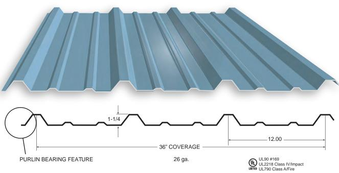
PBR Panel -- a higher-ribbed profile that is ideal for pre-engineered metal buildings. R-panels offer a high-strength, attractive profile and long-lasting performance. Manufactured in 26 ga. and 24 ga., and available in 22 ga. by special order. Minimum recommended slope is 1:12 with sealant.
