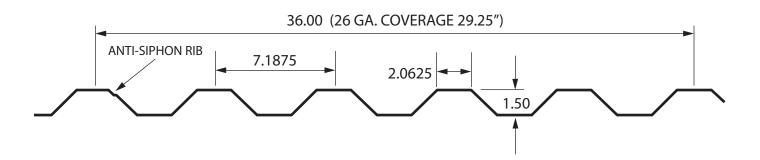
The MPI 7.2 Panel is one of the most versatile and economical products for commercial, industrial, and architectural applications. With a strong industrial aesthetic and it's sturdy symmetrical rib, the 7.2 Panel offers excellent spanning and cantilever capabilities, and can be installed vertically or horizontally.
