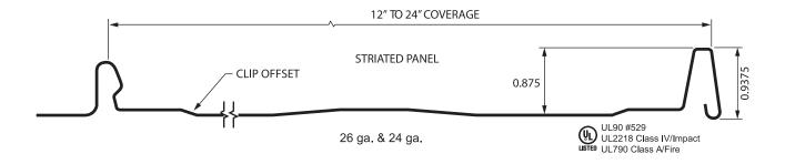
FF1 Panel -- is an economical snap-together panel with a 1" standing seam for use over a solid deck. Panels are installed by using a pancake fastener in the panel's fastener flange. Available in 26 ga. and 24 ga. Minimum recommended slope is 3:12. Pan striations required for all 26 ga. panels.
