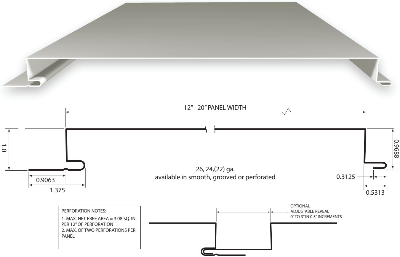
FP1-Panel -- is a maintenance-free prefinished panel for open spans. FP1-panel is a versatile panel for soffit, fascia, liner and ceiling applications. Adjustable configuration from flush to 3" reveal. Panel offered in smooth, grooved or perforated configurations.
