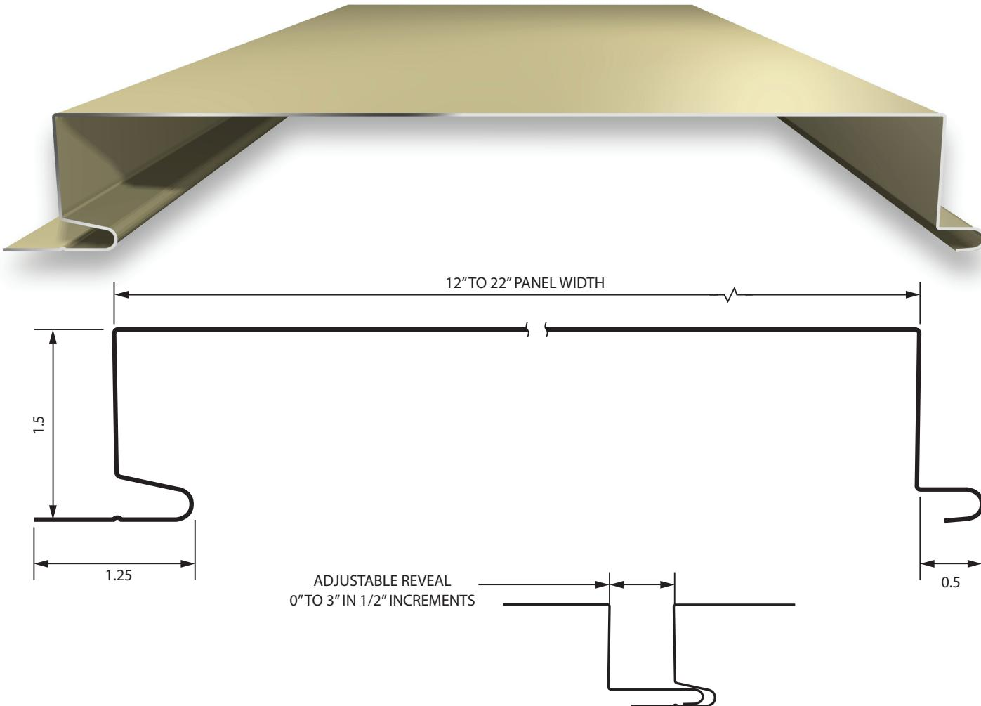
FP15-Panel -- is a maintenance-free prefinished panel for open spans. FP15-panel is a versatile panel for soffit, fascia, liner and ceiling applications. Adjustable configuration from flush to 3" reveal with 1½" depth. Panel offered in smooth, grooved or perforated configurations.
