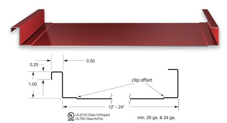
LF1 Panel -- is an architectural flat pan panel with a 1" standing seam that is mechanically seamed. Panels are typically used over a solid deck, but can be used over closely spaced open purlins. Panels are available in both 26 ga. and 24 ga. and include clip offsets. Minimum recommended slope is 2:12. Pan striations required for all 26 ga. panels.
