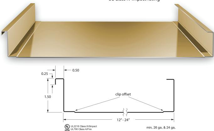
LF15 Panel -- is an architectural flat pan panel with a  $1\frac{1}{2}$ " standing seam that is mechanically seamed. Panels are typically used over a solid deck, but can be used over closely spaced open purlins. Panels are available in both 26 ga. and 24 ga. Minimum recommended slope is 1:12. Pan striations required for all 26 ga. panels.
