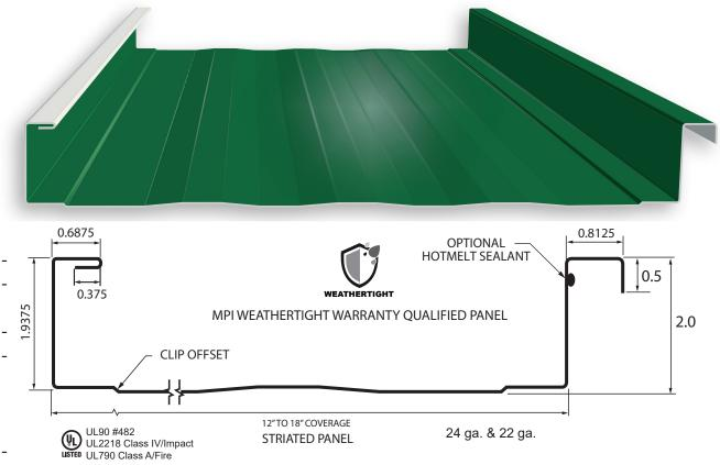
LF2 Panel -- is an architectural/structural standing seam roof system for use over open purlins or a solid deck. The panel features a 2" standing seam that is mechanically seamed in a single or double lock configuration. Minimum recommended slope is 0.5:12. Panels can be ordered as smooth, striated or two-bead.
