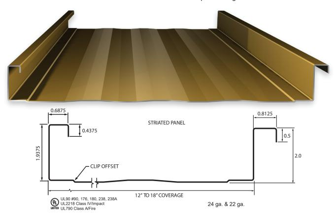
LF2A Panel -- is a mechanically-seamed architectural/structural standing seam roof system for use over open purlins or a solid deck. This panel features a return leg on both the male and female seams that help increase strength and wind uplift resistance. Minimum recommended slope is 0.5:12. Panels can be ordered as smooth, striated or two-bead.
