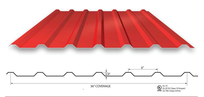
M-Panel -- a stiffer profile panel that is ideal for liner panels for pre-engineered metal buildings. M-panels offer high-strength with ribs 6" on center for durable performance. Manufactured in 26 ga. and 24 ga. Minimum slope, 3:12.
