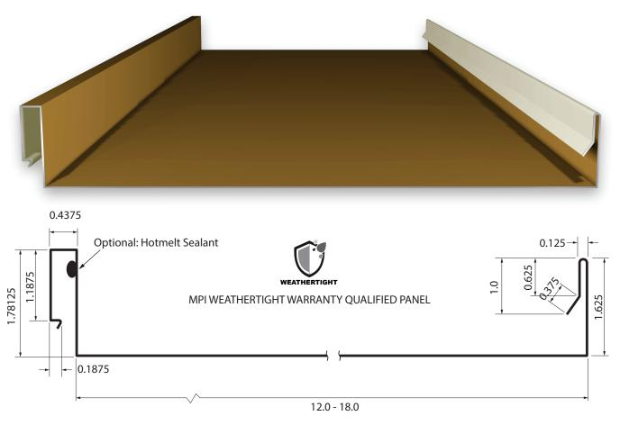
SL175 Panel is an exceptional architectural/structural standing seam roof system that may be utilized in a variety of roof, mansard, and fascia applications. The design allows for application over a variety of solid substrates as well as over open purlins. The SL175 features hidden clips and a snap-lock seam which eliminates the need of jobsite seaming. Minimum slope, 2:12.
