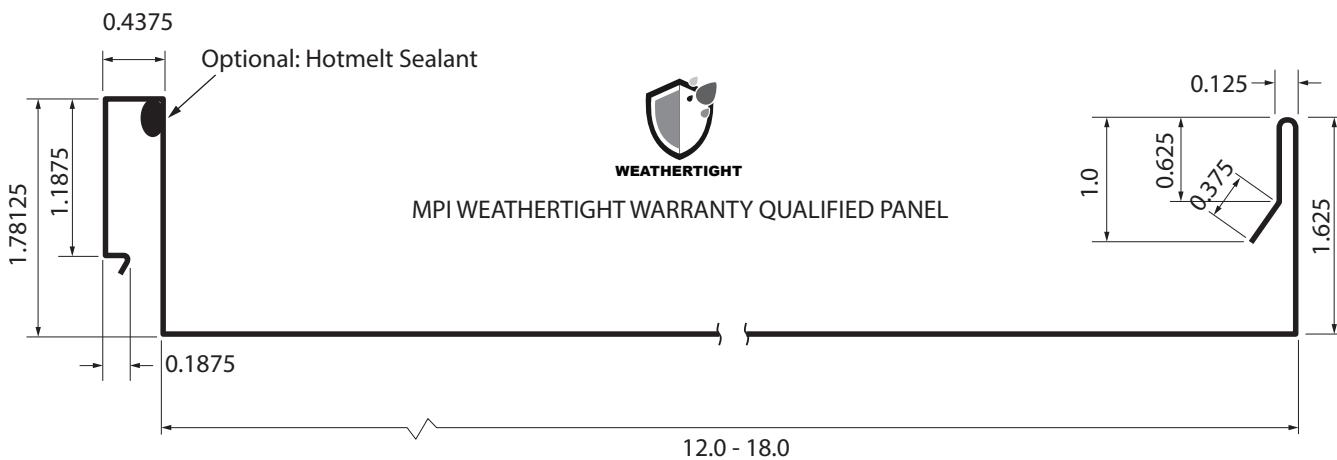
SL175 Panel is an exceptional architectural/structural standing seam roof system that may be utilized in a variety of roof, mansard, and fascia applications. The design allows for application over a variety of solid substrates as well as over open purlins. The SL175 features hidden clips and a snap-lock seam which eliminates the need of jobsite seaming. Minimum slope, 2:12.
