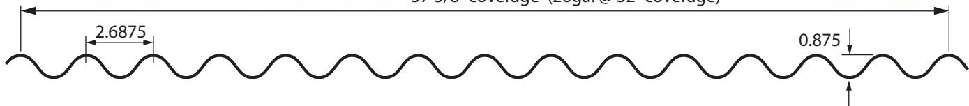
7/8" Corrugated Panel - Structurally strong and incredibly impact resistant, MPI's 7/8" Corrugated Panel is an excellent choice for exterior roofing, siding applications or interior projects. The 7/8" Corrugated Panel is an economical, structural, exposed fastener metal roof and wall panel. Recommended minimum slope, 3:12.
